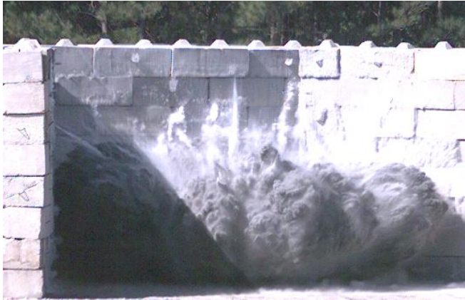
Figure 4. Frame of high-speed video of blast test.
