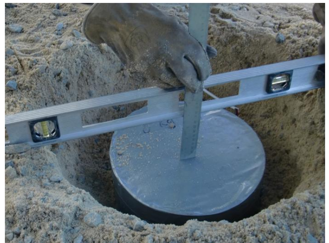
Figure 3. Mine emplacement with 4" soil overburden.
